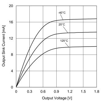
Figure 13. Output Sink Current vs Output Voltage (V<sub>DD</sub>=1.8 V)
