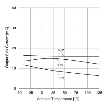
Figure 16. Output Sink Current vs Ambient Temperature (V<sub>OUT</sub>=V<sub>SS</sub>+0.4 V)
