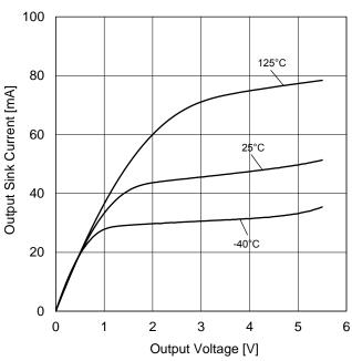
Figure 14. Output Sink Current vs Output Voltage (V<sub>DD</sub>=3.0 V)
