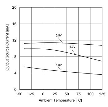
Figure 12. Output Source Current vs Ambient Temperature ( $V_{OUT}$ = $V_{DD}$ -0.4 V)
