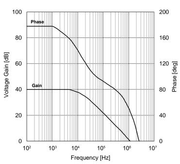
Figure 29. Voltage Gain • Phase vs Frequency (V<sub>DD</sub>=3.0 V)
