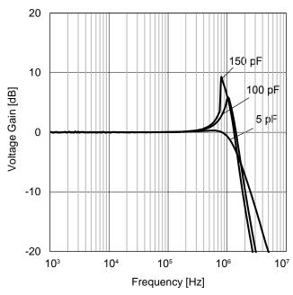
Figure 35. Voltage Gain vs Frequency  $(V_{DD}=3.0 \text{ V}, \text{Gv}=0 \text{ dB})$
