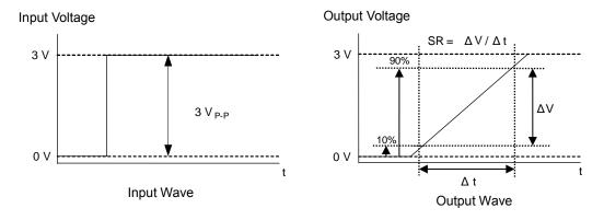
Figure 32. Slew Rate Input and Output Wave
