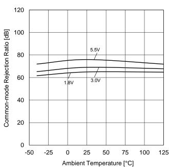
Figure 25. Common-mode Rejection Ratio vs Ambient Temperature
