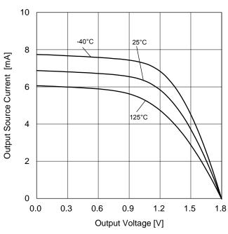
Figure 9. Output Source Current vs Output Voltage (V<sub>DD</sub>=1.8 V)
