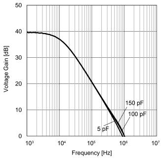
Figure 34. Voltage Gain vs Frequency (V<sub>DD</sub>=3.0 V, G<sub>V</sub>=40 dB)
