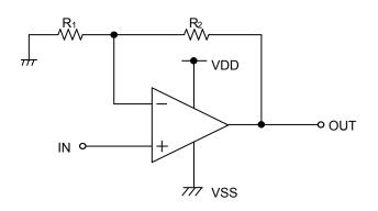
Figure 44. Non-inverting Amplifier Circuit
