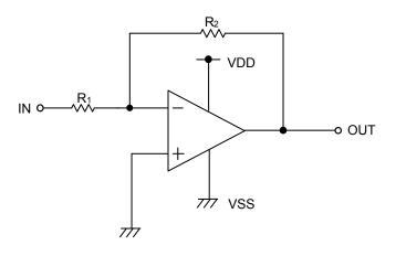
Figure 43. Inverting Amplifier Circuit
