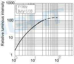
Forward Current I<sub>F</sub> (mA) Radiation Diagram Ta=25°C
