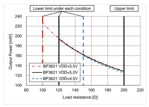
Figure 2. Output Power vs Load resistance
