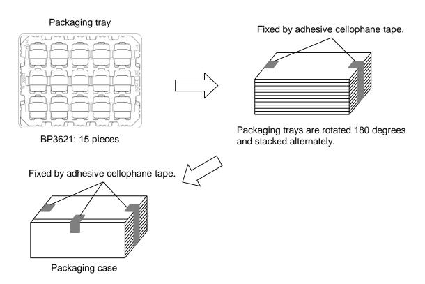
Figure 12. Packing Method
