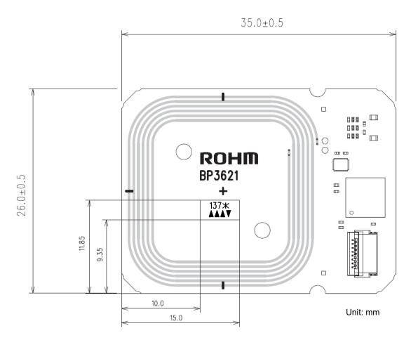
Figure 10. PCB Marking Specification
