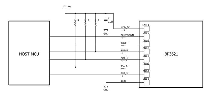
Figure 11. Reference Circuit Diagram
