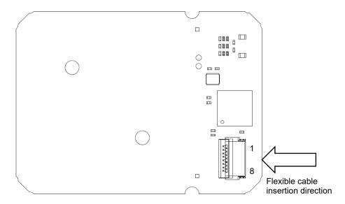
Figure 9. Pin Number (flexible cable connector)
