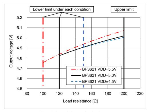
Figure 3. Output Voltage vs Load resistance
