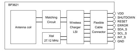
Figure 1. Block Diagram
