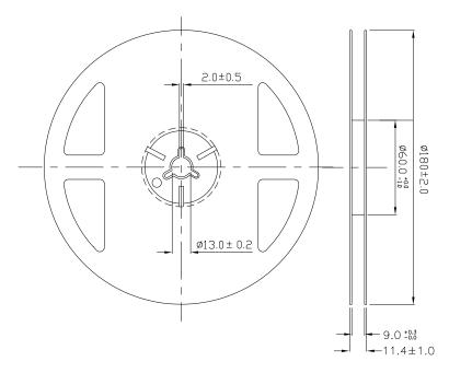
Note: The tolerances unless mentioned is ±0.1mm ,Unit = mm
