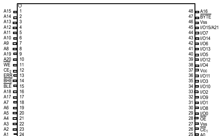
Figure 5. 48-pin TSOP I Pinout (Dual Chip Enable with ERR) – CY62177GE30 [8, 9]
