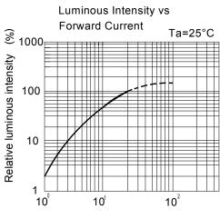
Forward Current  $I_{E}(mA)$ Ta=25°C Radiation Diagram ٥° 10° 20°
