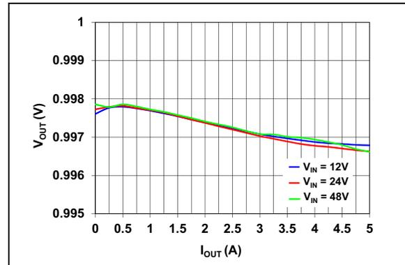
**FIGURE 2-5:** Output Voltage vs. Output Current ( $V_{OUT} = 1V$ ).
