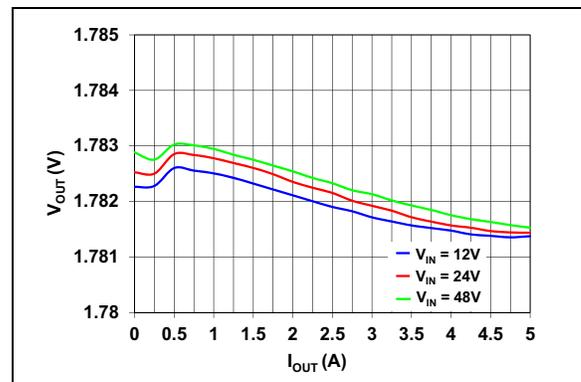
**FIGURE 2-6:** Output Voltage vs. Output Current ( $V_{OUT} = 1.8V$ ).
