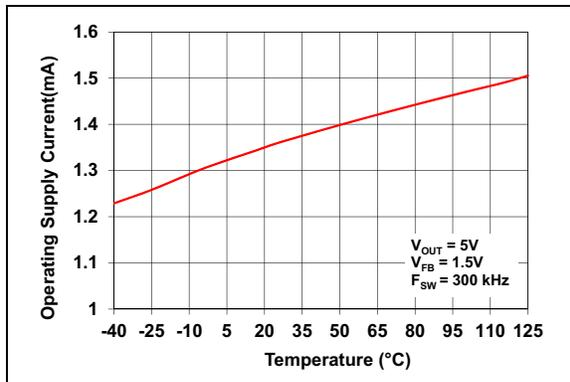
**FIGURE 2-14:**  $V_{IN}$  Operating Supply Current vs. Temperature.
