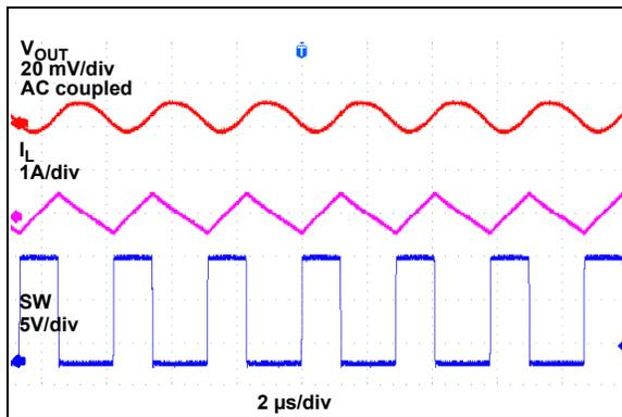
**FIGURE 2-32:** Switching Waveform ( $I_{OUT} = 0A$ ).
