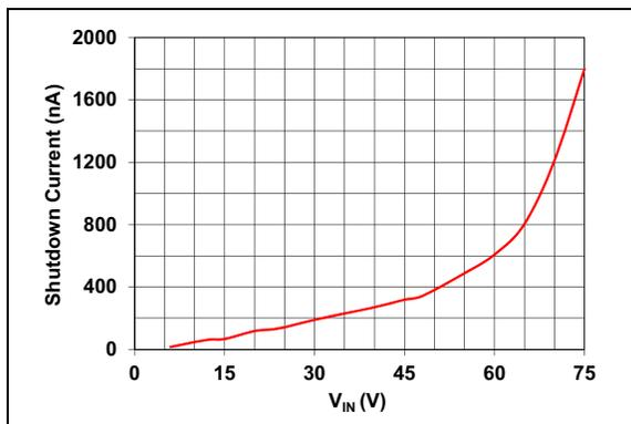
**FIGURE 2-15:**  $V_{IN}$  Shutdown Current vs. Input Voltage.
