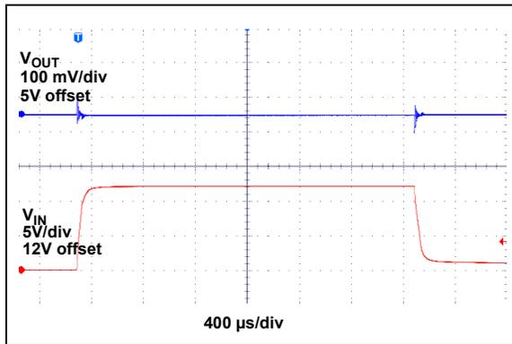
**FIGURE 2-43:** Line Transient Response (12V to 24V).
