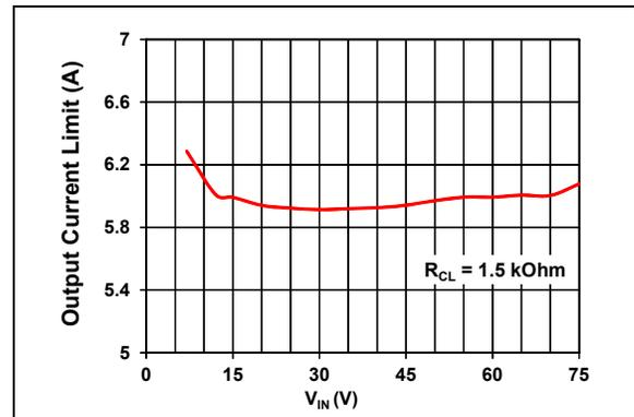
**FIGURE 2-23:** Output Current Limit vs. Input Voltage.
