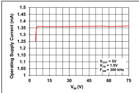
**FIGURE 2-13:**  $V_{IN}$  Operating Supply Current vs. Input Voltage.
