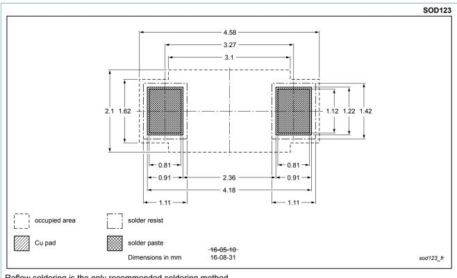
Reflow soldering is the only recommended soldering method.
