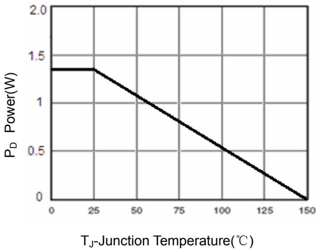
Figure 3 Power Dissipation
