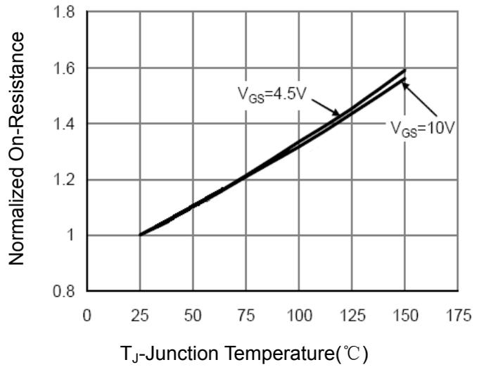
**Figure 8 Drain-Source On-Resistance**
