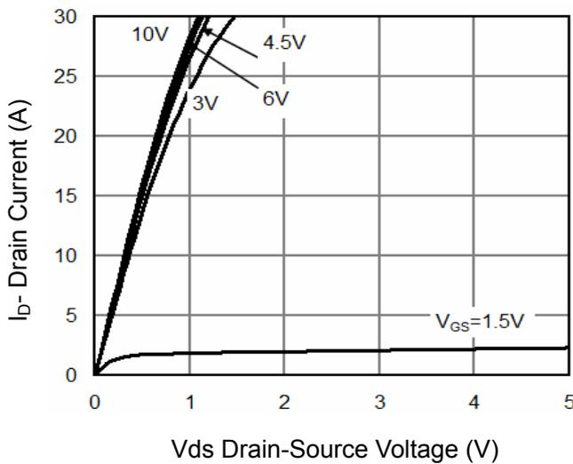
Figure 5 Output Characteristics
