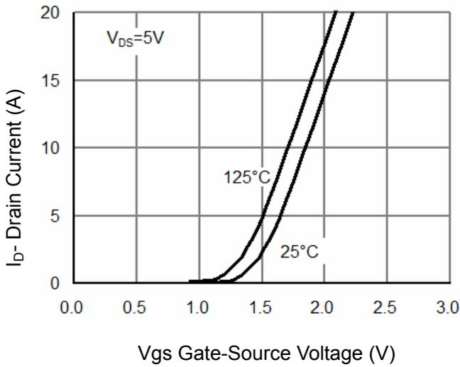
**Figure 7 Transfer Characteristics**
