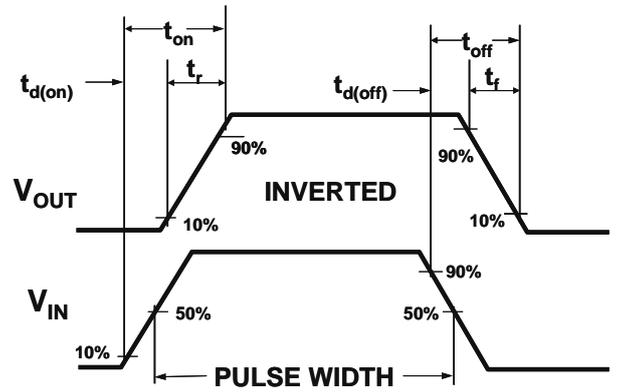
Figure 2: Switching Waveforms
