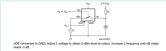
Fig. 17. Test circuit for measuring the frequency response when channel is in ON-state
