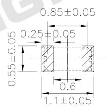
**Note:** The tolerances unless mentioned is  $\pm 0.1$ mm ,Unit = mm Suggested pad dimension is just for reference only. Please modify the pad dimension based on individual need.
