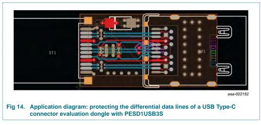
Since the SuperSpeed TX/RX lines are separated by GND or VBUS from the Hi-Speed lines, PESD1USB3S makes it easy to achieve same signal lengths, straight routing, and optimal positioning for ESD protection directly at the connector.
