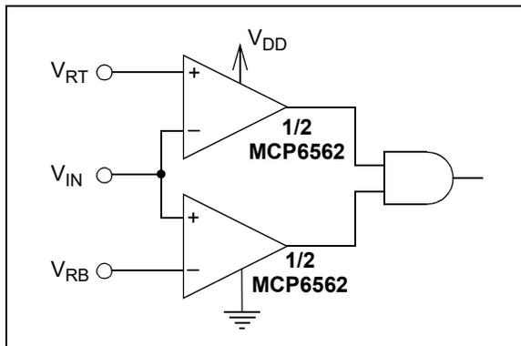
**FIGURE 4-13:** Windowed Comparator.
