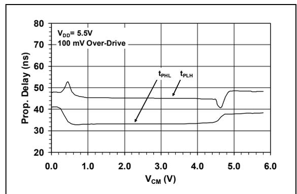
**FIGURE 2-30:** Propagation Delay vs. Common-Mode Input Voltage.
