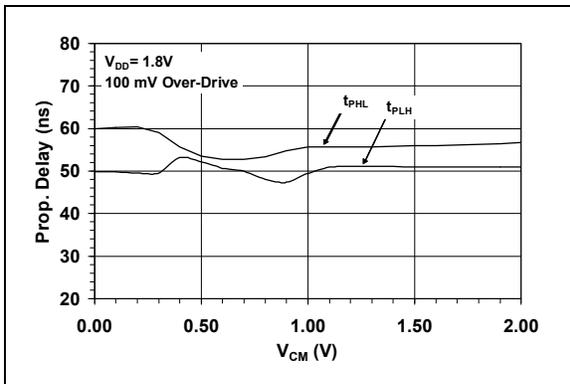
**FIGURE 2-27:** Propagation Delay vs. Common-Mode Input Voltage.
