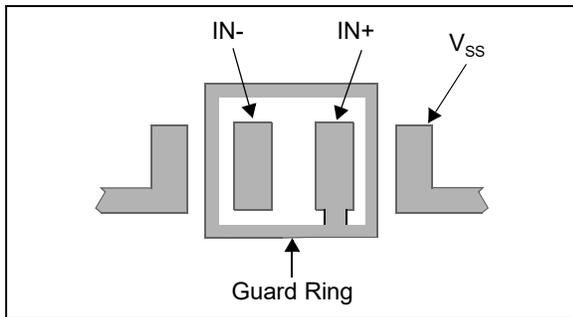
**FIGURE 4-9:** Example Guard Ring Layout for Inverting Circuit.
