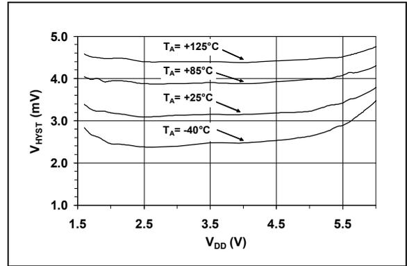
**FIGURE 2-16:** Input Hysteresis Voltage vs. Supply Voltage vs. Temperature.
