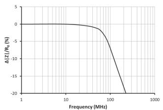
Typical high frequency characteristics for WMHP35-220R. Self resonant frequency is 1GHz.
