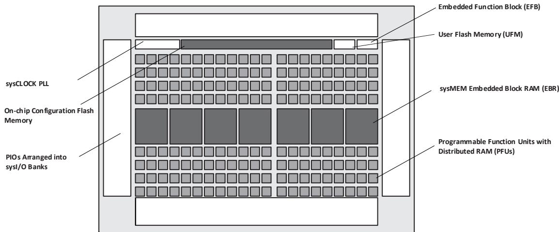
Note: MachXO2-256, and MachXO2-640/U are similar to MachXO2-1200. MachXO2-256 has a lower LUT count and no PLL or EBR blocks. MachXO2-640 has no PLL, a lower LUT count and two EBR blocks. MachXO2-640U has a lower LUT count, one PLL and seven EBR blocks.
