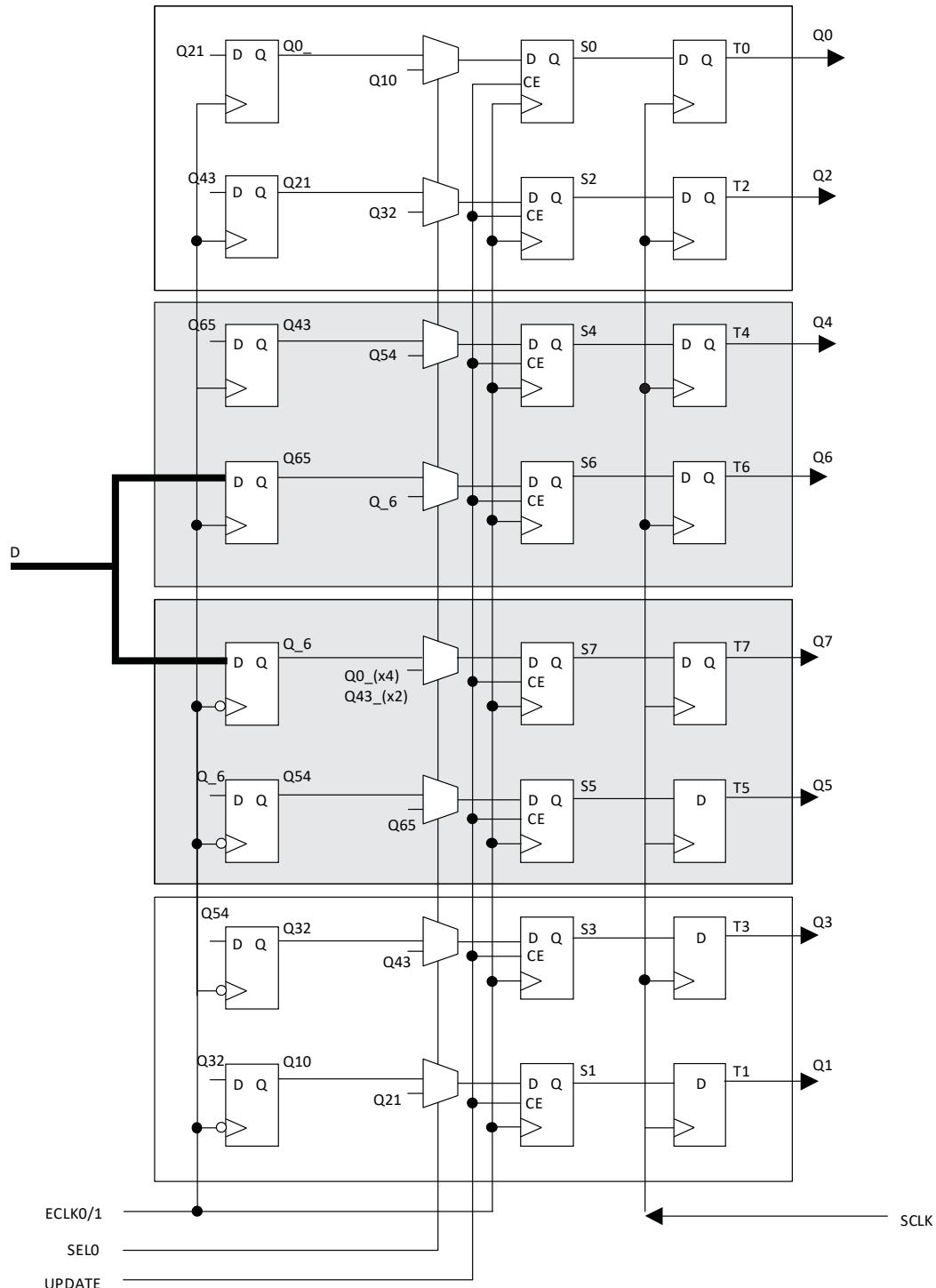
**Figure 2.16. Input Gearbox**
