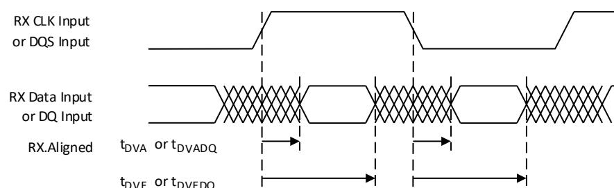
Figure 3.5. Receiver RX.CLK.Aligned and MEM DDR Input Waveforms
