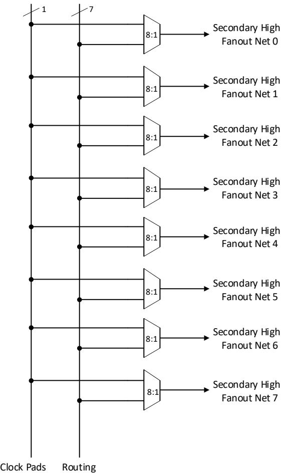
Figure 2.6. Secondary High Fanout Nets for MachXO2 Devices
