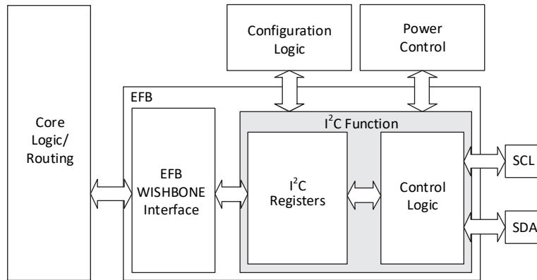
Figure 2.21. I<sup>2</sup>C Core Block Diagram
