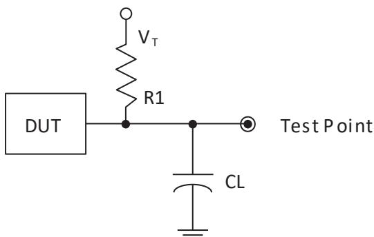
**Figure 3.13. Output Test Load, LVTTL and LVCMOS Standards**
