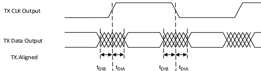
**Figure 3.7. Transmitter TX.CLK.Aligned Waveforms**
