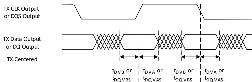
**Figure 3.8. Transmitter TX.CLK.Centered and MEM DDR Output Waveforms**
