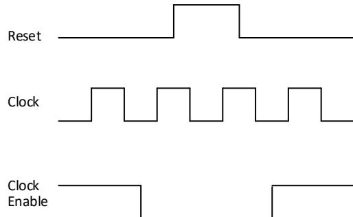
**Figure 2.10. EBR Asynchronous Reset (Including GSR) Timing Diagram**
