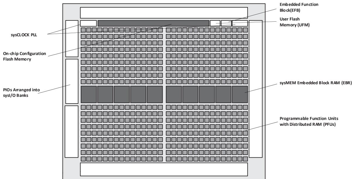
Note: MachXO2-1200U, MachXO2-2000/U and MachXO2-7000 are similar to MachXO2-4000. MachXO2-1200U and MachXO2-2000 have a lower LUT count, one PLL, and eight EBR blocks. MachXO2-2000U has a lower LUT count, two PLLs, and 10 EBR blocks. MachXO2-7000 has a higher LUT count, two PLLs, and 26 EBR blocks.
