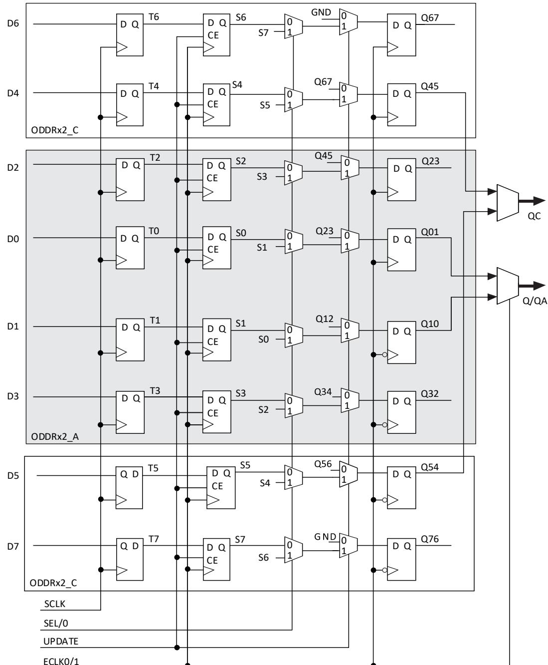
**Figure 2.17. Output Gearbox**
